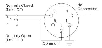
Figure 15 Timer Connections Contacts shown with TIMER OFF
