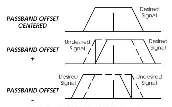
FIGURE 9 PASSBAND OFFSET Operation
